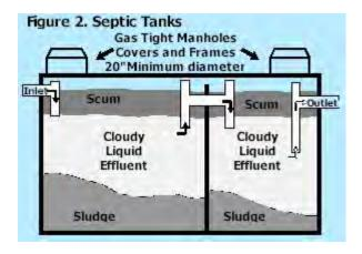
The overflow of solid material into the soil absorption area should be avoided because it will clog soil pores in the absorption area and result in system failure. Two factors contribute to solid material overflow: bacterial deficiency and failure to have sludge accumulations removed periodically.
