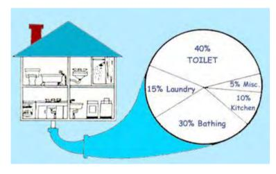
Septic systems are called upon to receive and process household wastewater from toilets, showers, washing machines, sinks and garbage disposal units (see Figure 1). Their efficiency is dependent upon their design, proper installation, and maintenance program. Failure in any one of these areas can lead to improper operation, which can create a health hazard and a potential financial burden.
