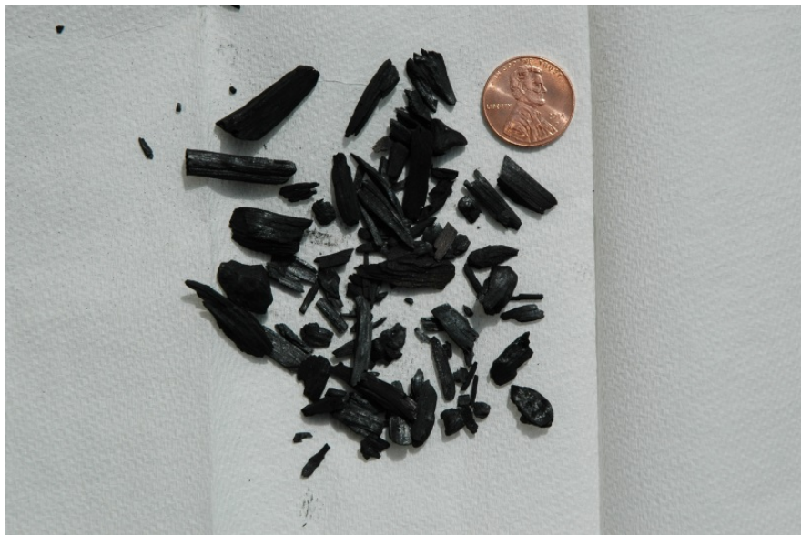
Figure 1: Photograph of the Biochar Particles Mixed with Field and Mine Soil (Penny in Photograph Provided for Scale)
