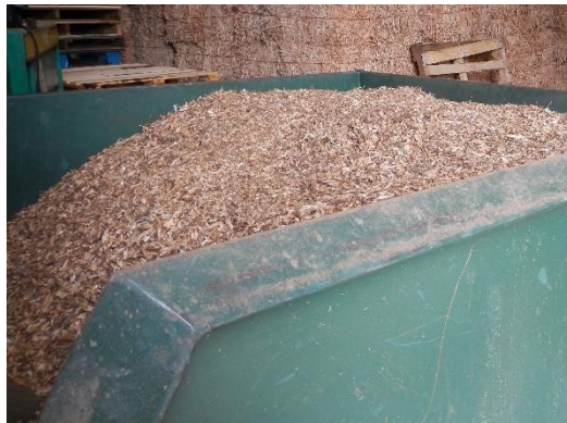
Figures 12 a,b. Finished screened feedstock and partially filled hook-lift container of finished feedstock.
