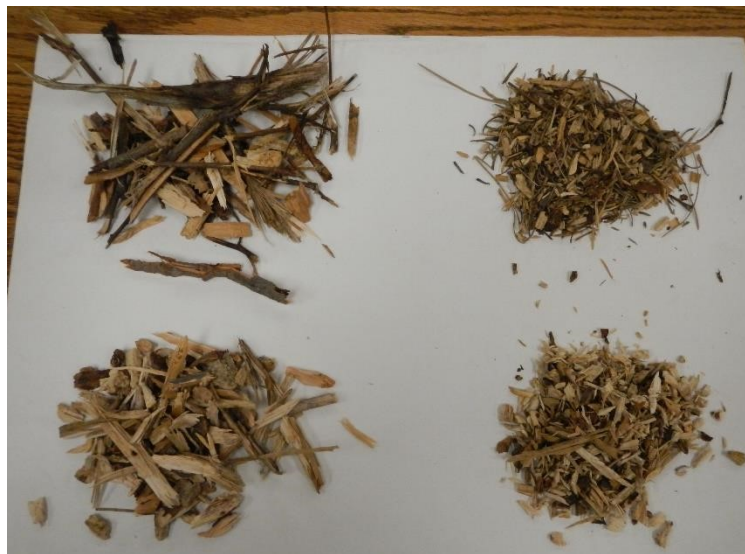
Figure 6. Recutting overs with Forest Concepts Crumbler® using 3/8 inch cutter set. Top left is overs from original raw biomass. Top right is accepts (3/8 minus) from raw biomass. Lower left is overs retained on 3/8 screen after recutting. Lower right is accepts (3/8 minus) from recut material. Pile sizes are for photo only and not representative of the mass percentages.
