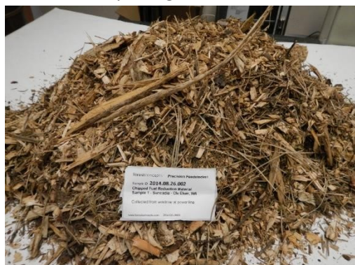
Figures 2a,b. Sample of fuel reduction chips and dividing into sub-samples for analysis.
