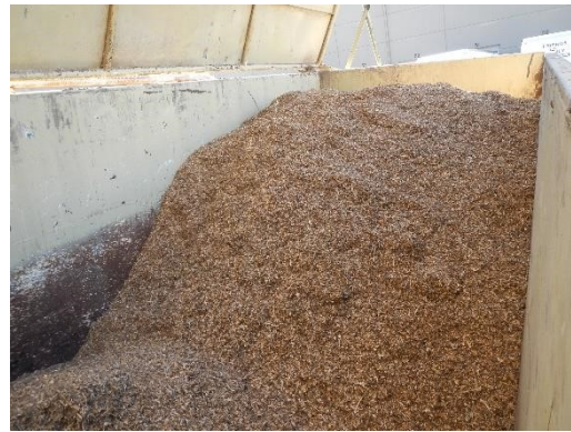
Figures 12 a,b. Finished screened feedstock and partially filled hook-lift container of finished feedstock.
