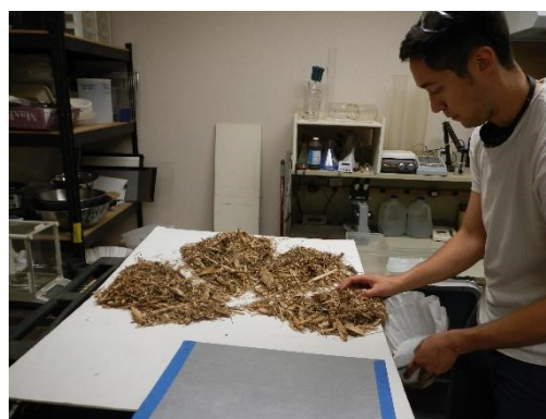
Figures 2a,b. Sample of fuel reduction chips and dividing into sub-samples for analysis.
