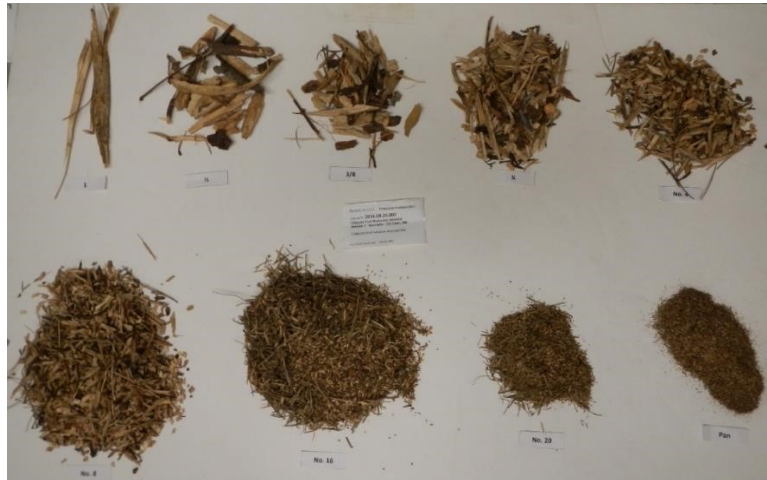
Figure 4. Particles retained on each sieve for sample no. 2014.08.26.002. Pile sizes include the entire mass captured on each screen.
