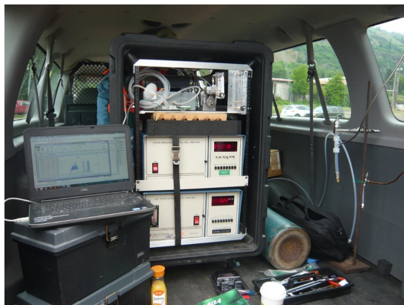
Figure 1. Photograph of instrumentation and laptop recording data from pyrolysis emissions testing in Bingen, WA.
