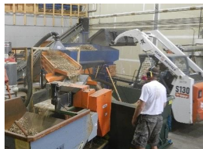
Figures 9 a,b,c. Raw biomass pile with tarp, skid-steer loader bucket of raw biomass, loader filling the hopper. (Note that colors shift between outdoor and indoor lighting.)
