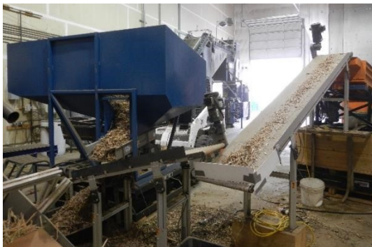
Figures 10 a,b. Hopper outfeed and elevator conveyor. Rocks and debris removed from infeed and screen deck by hand. Note pine cones rolled back off the lower end of the sloped conveyor.
