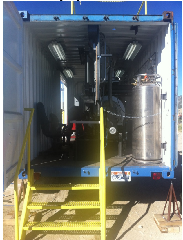
Figure 2 – The Amaron Energy Rotary Pyrolysis Reactor
